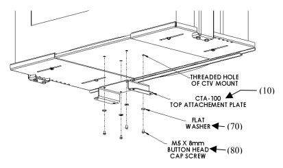
Figure 6. Install Top Attachment Plate
